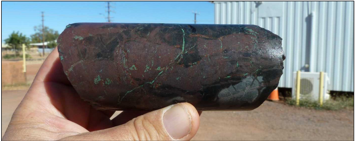
Figure 1 – Strongly mineralised hematite-chlorite breccia in drill core from BBDD-2, Bluebird Prospect, Tennant Creek
