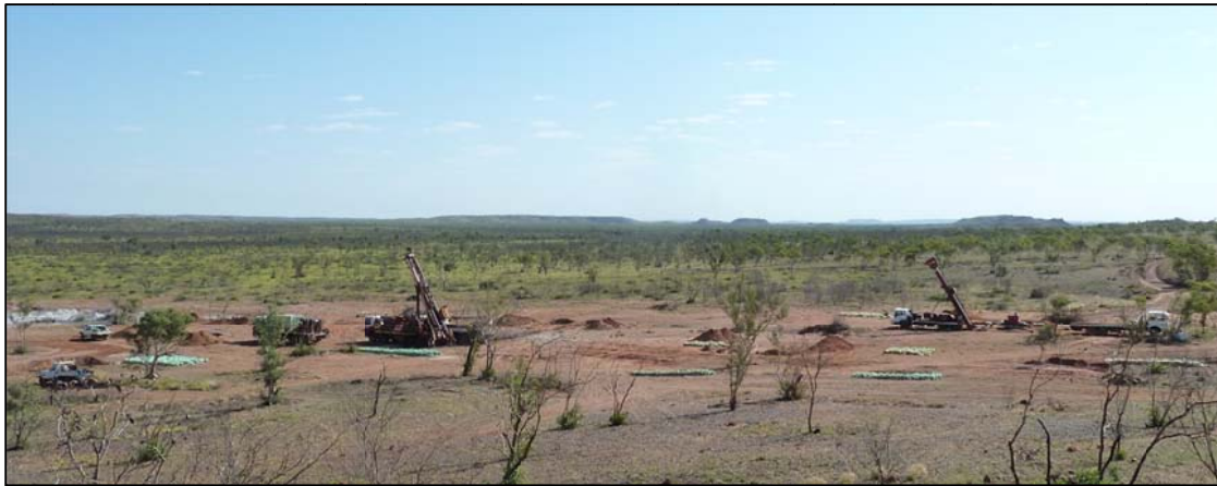
Figure 1 –Bluebird Prospect, Tennant Creek, looking south west. Diamond rig (right) and RC rig (left) in action on phase II drilling.
