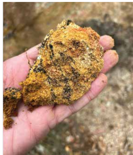
A sample of rare earths-enriched clay taken from the Caldeira project in Brazil
